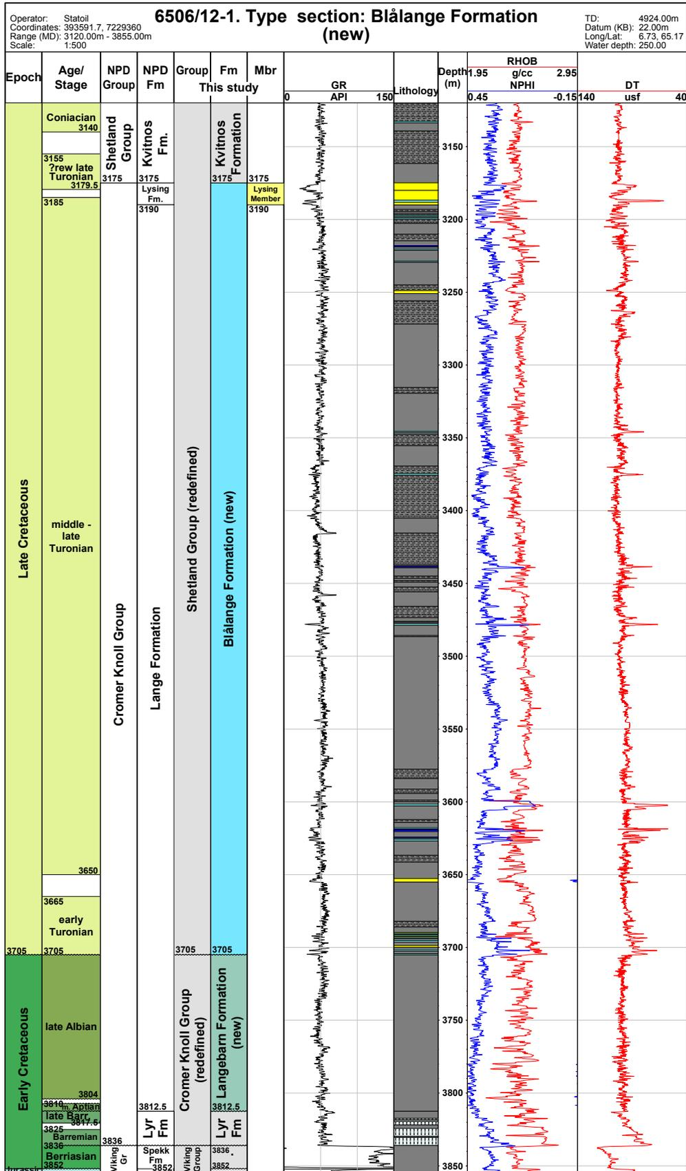
Figure 3.14. Well logs and lithology section for the Blålänge Formation in type well 6506/12-1, Norwegian Sea.
