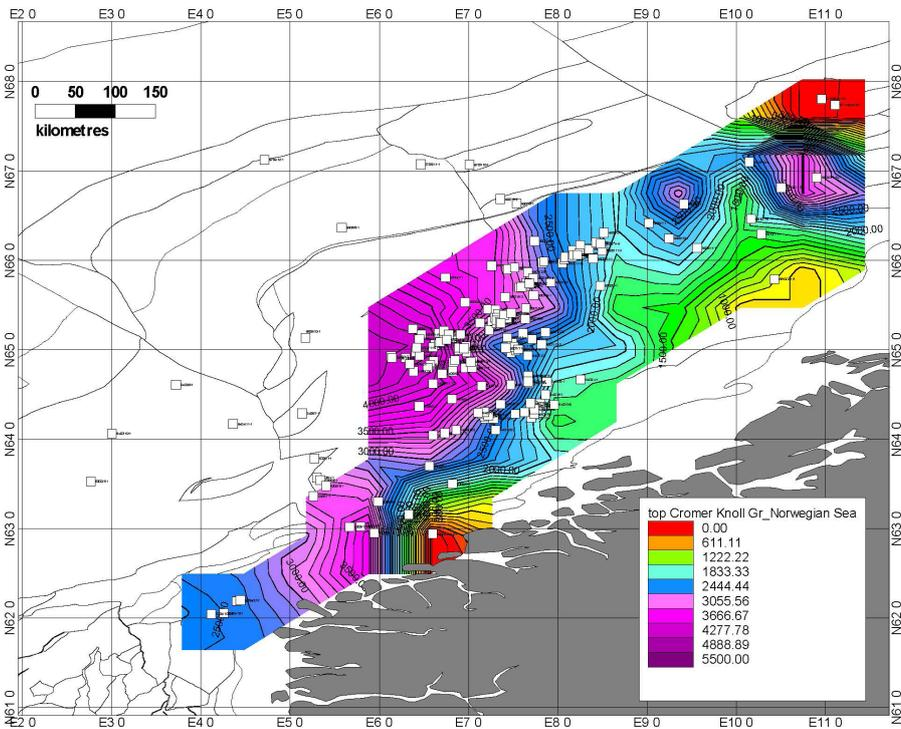
Figure 3.6. shows depth to the top of the Cromer Knoll Group (revised definition) in the Norwegian Sea based on released well data. This follows the revised definition that corresponds to the top Lower Cretaceous, and coincides with the level applied in the North Sea. The wells displayed are those that penetrated the group.
