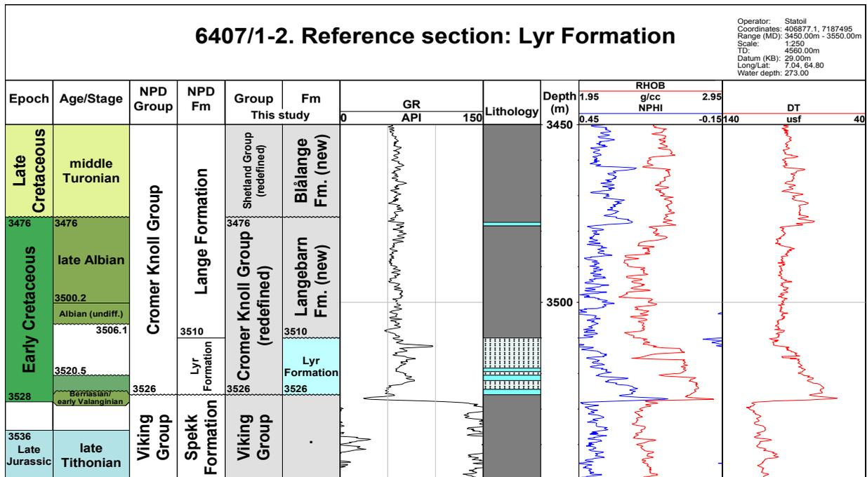
Figure 3.8. Well logs and lithology for the Lyr Formation in reference well 6407/1-2, Norwegian Sea.
