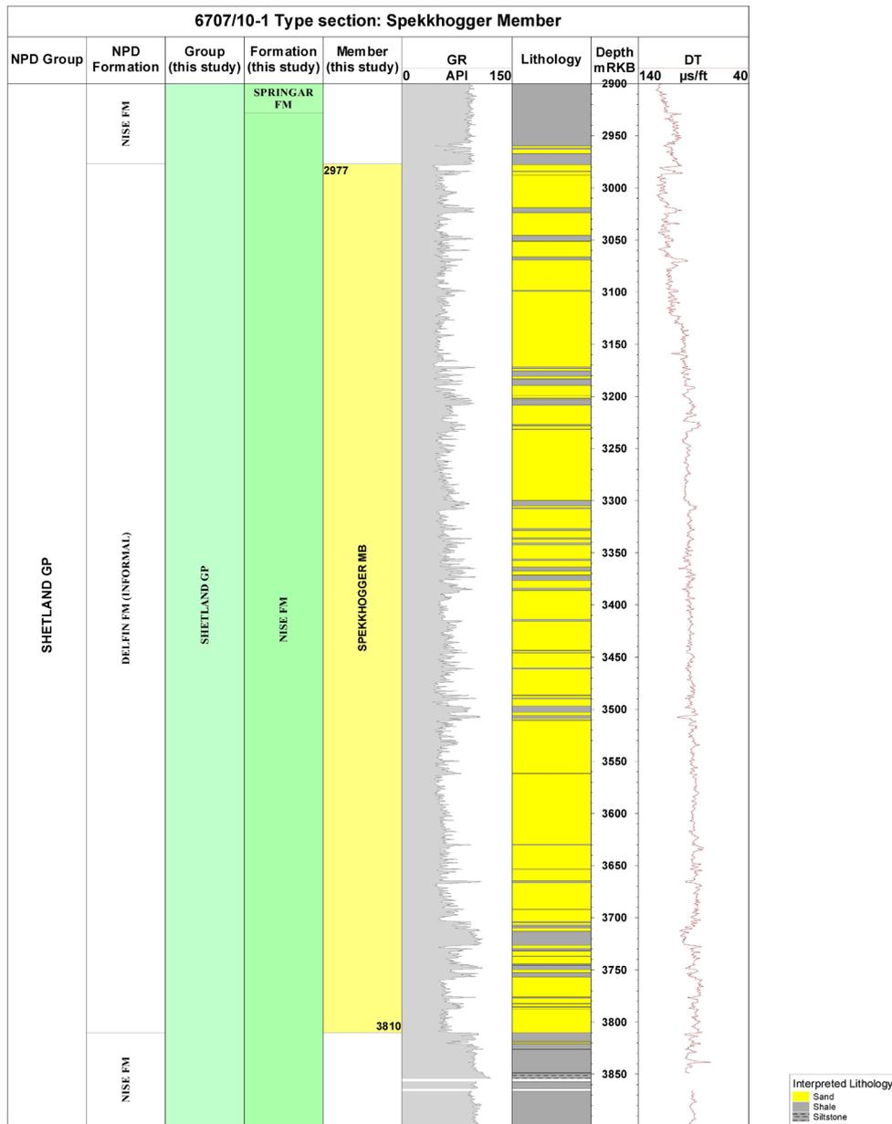
**Figure 3.34.** Well logs and lithology section for the Spekkhogger Member of the Nise Formation in type well 6707/10-1, Norwegian Sea.
