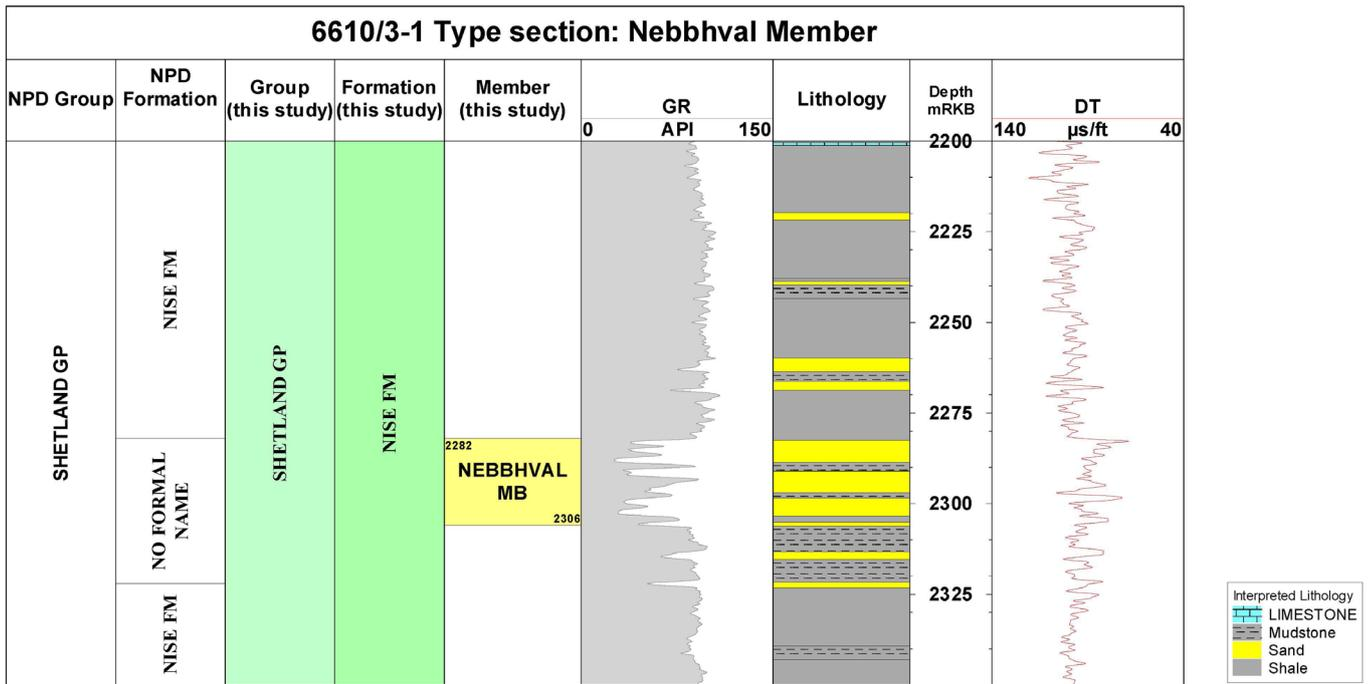
Figure 3.35. Well logs and lithology section for the Nebbhval Member of the Nise Formation in type well 6610/3-1, Norwegian Sea.
