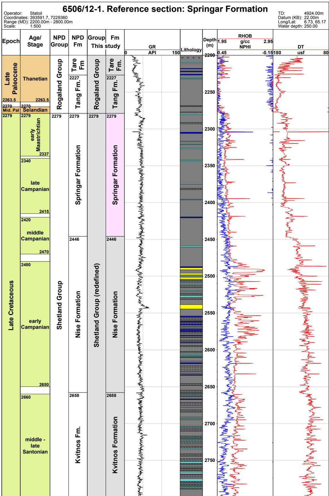
Figure 3.37. Well logs and lithology section for the Springar Formation in type well 6506/12-1, Norwegian Sea.
