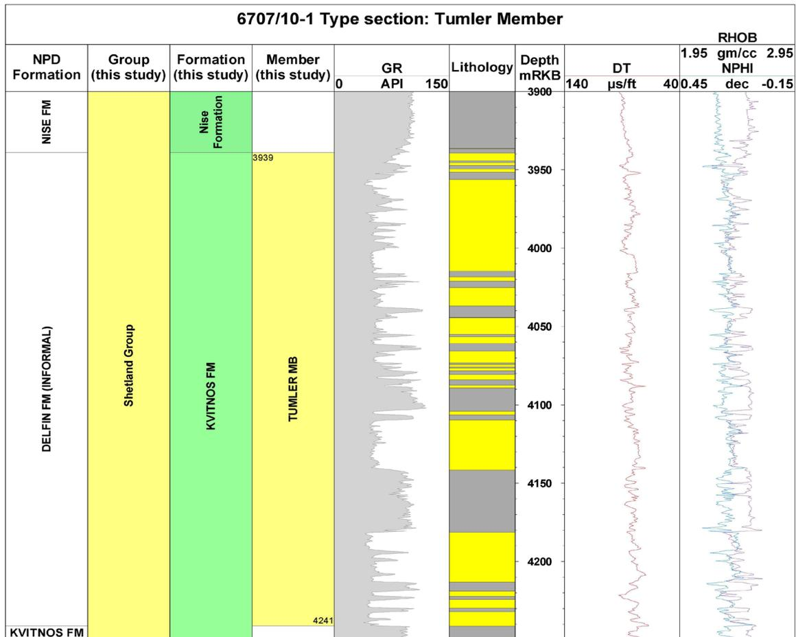
**Figure 3.29.** Well logs and lithology section for the Tumler Member of the Kvitnos Formation in type well 6707/10-1.
