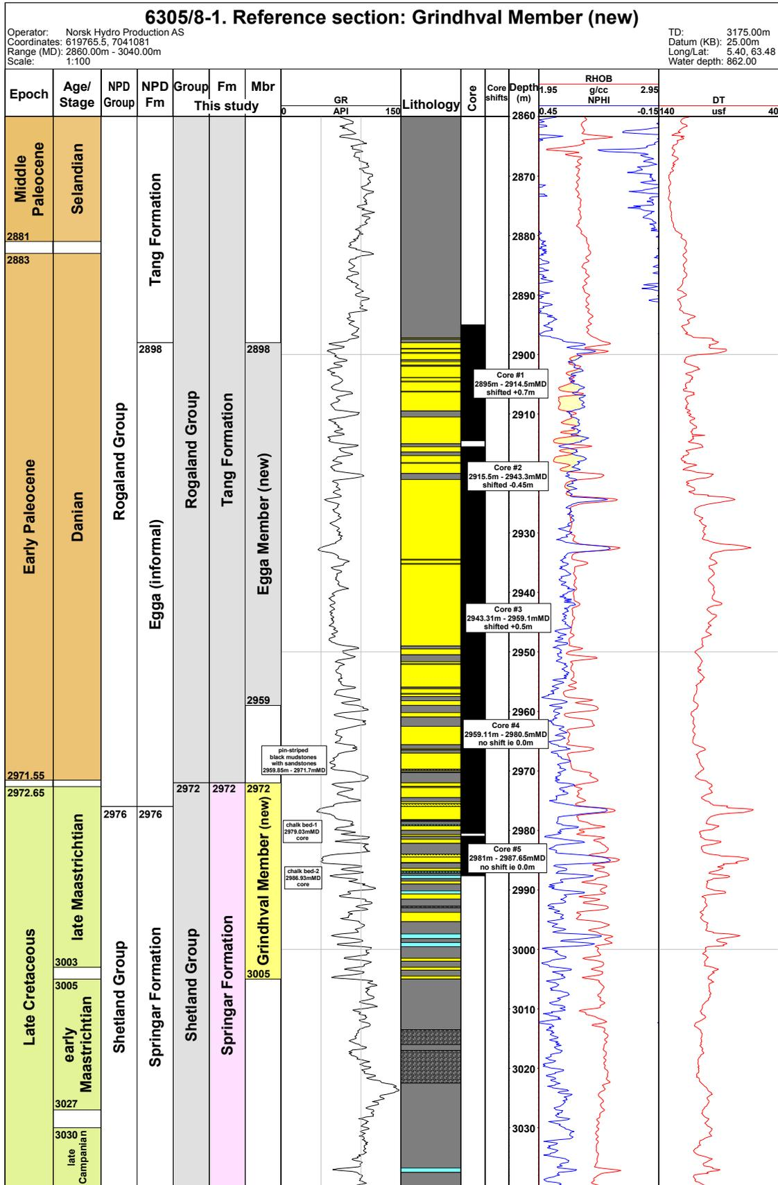
Figure 3.42. Well logs and lithology section for the Grindhval Member of the Springar Formation in reference well 6305/8-1, Norwegian Sea.
