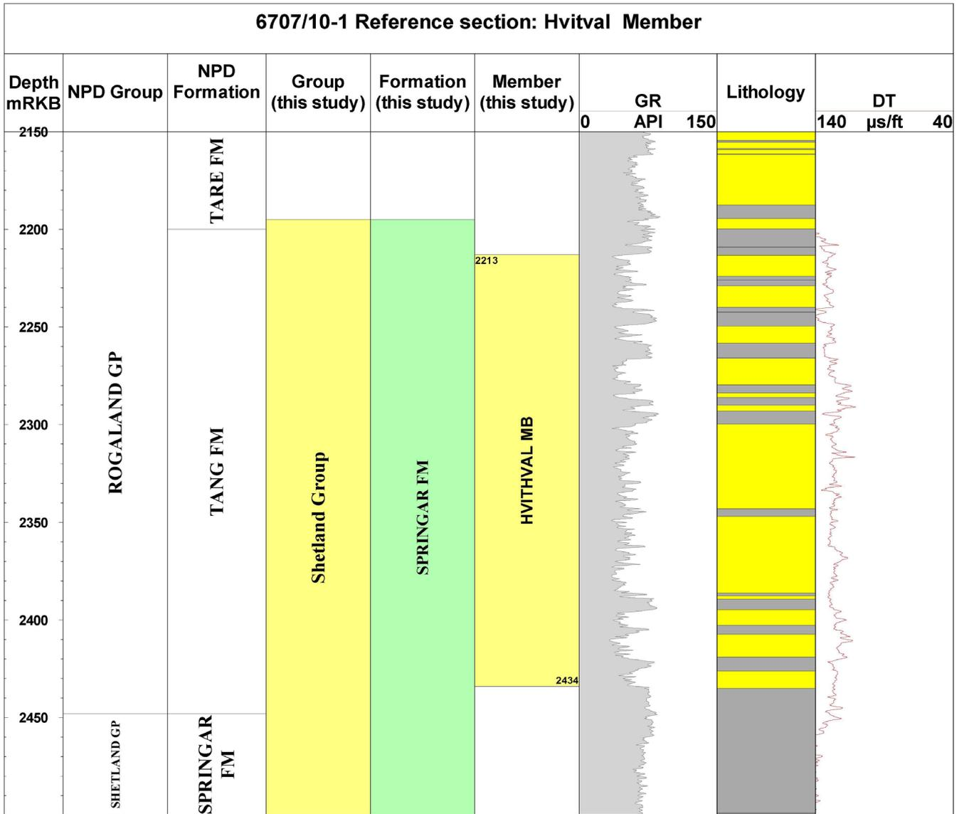
Figure 3.39. Well logs and lithology section for the Hvitval Member of the Springar Formation in reference well 6707/10-1, Norwegian Sea.
