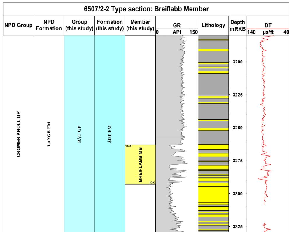
**Figure 3.20.** Well logs and lithology section for the Breiflabbb Member of the Blålänge Formation in type well 6507/2-2, Norwegian Sea.
