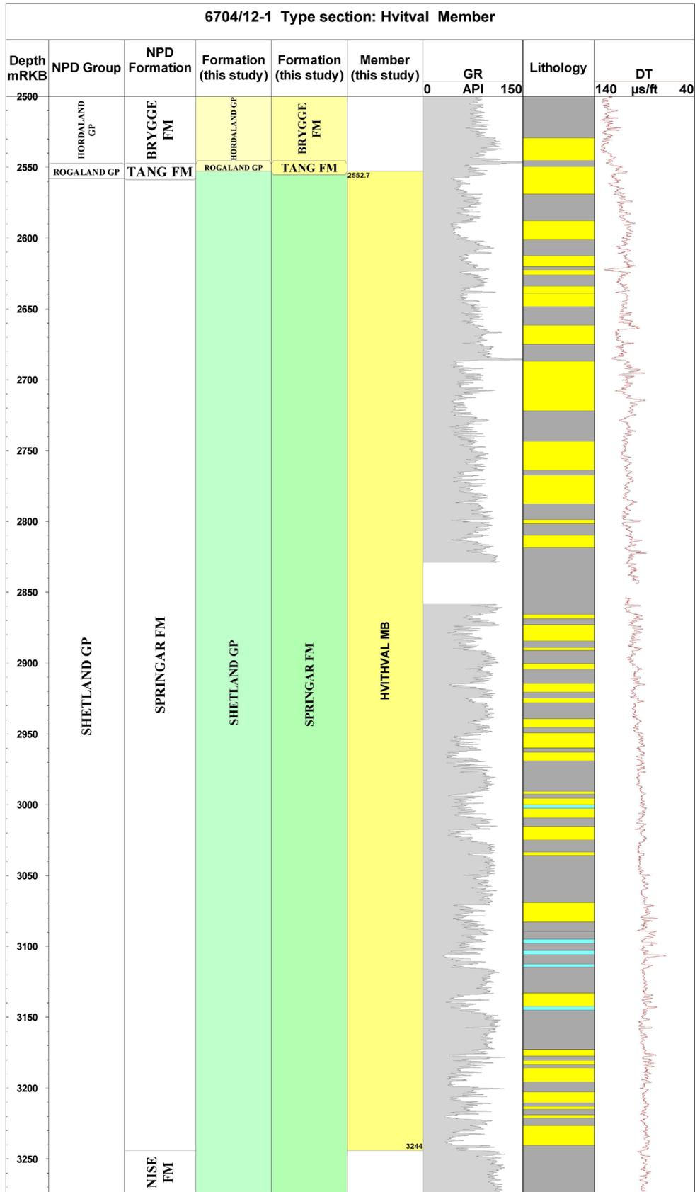
**Figure 3.38.** Well logs and lithology section for the Hvitval Member of the Springar Formation in type well 6704/12-1, Norwegian Sea.
