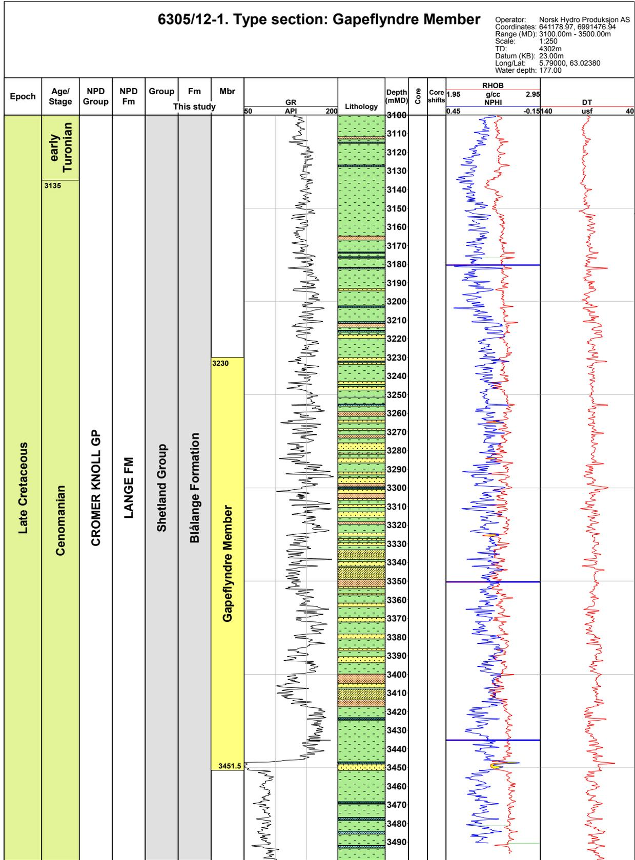
Figure 3.18. Well logs and lithology section for the Gapeflyndre Member of the Blålänge Formation in type well 6305/12-1, Norwegian Sea.
