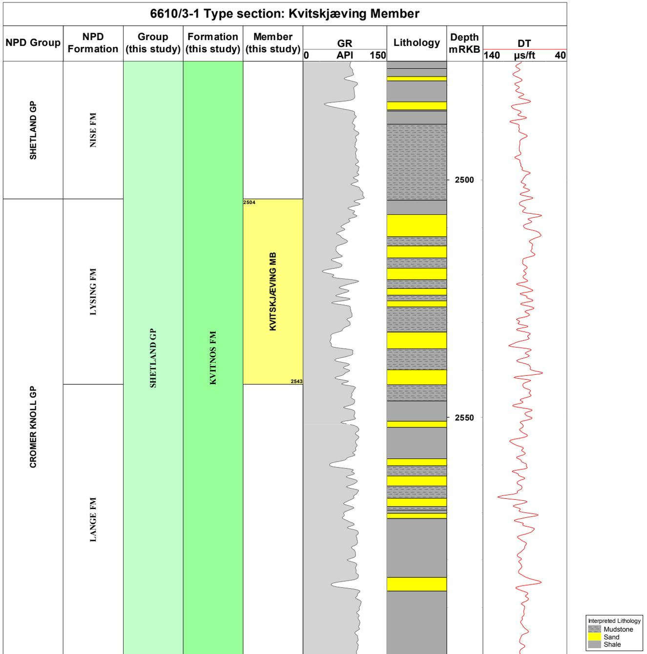
**Figure 3.28.** Well logs and lithology section for the Kvitskjæving Member of the Kvitnos Formation in type well 6610/3-1, Norwegian Sea.
