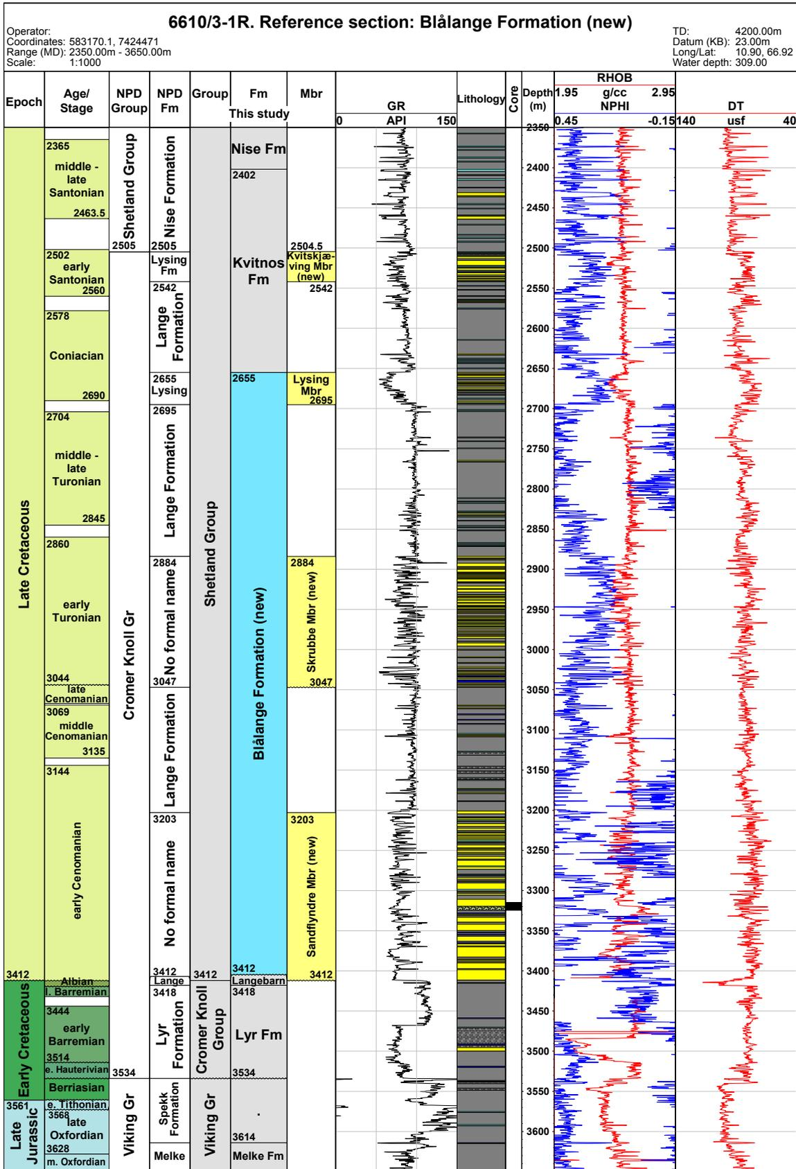
Figure 3.16. Well logs and lithology section for the Blålange Formation in type well 6610/3-1R, Norwegian Sea.
