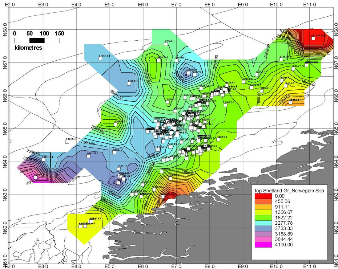
Figure 3.11. Depth to top of the Shetland Group in the Norwegian Sea based on released well data.
