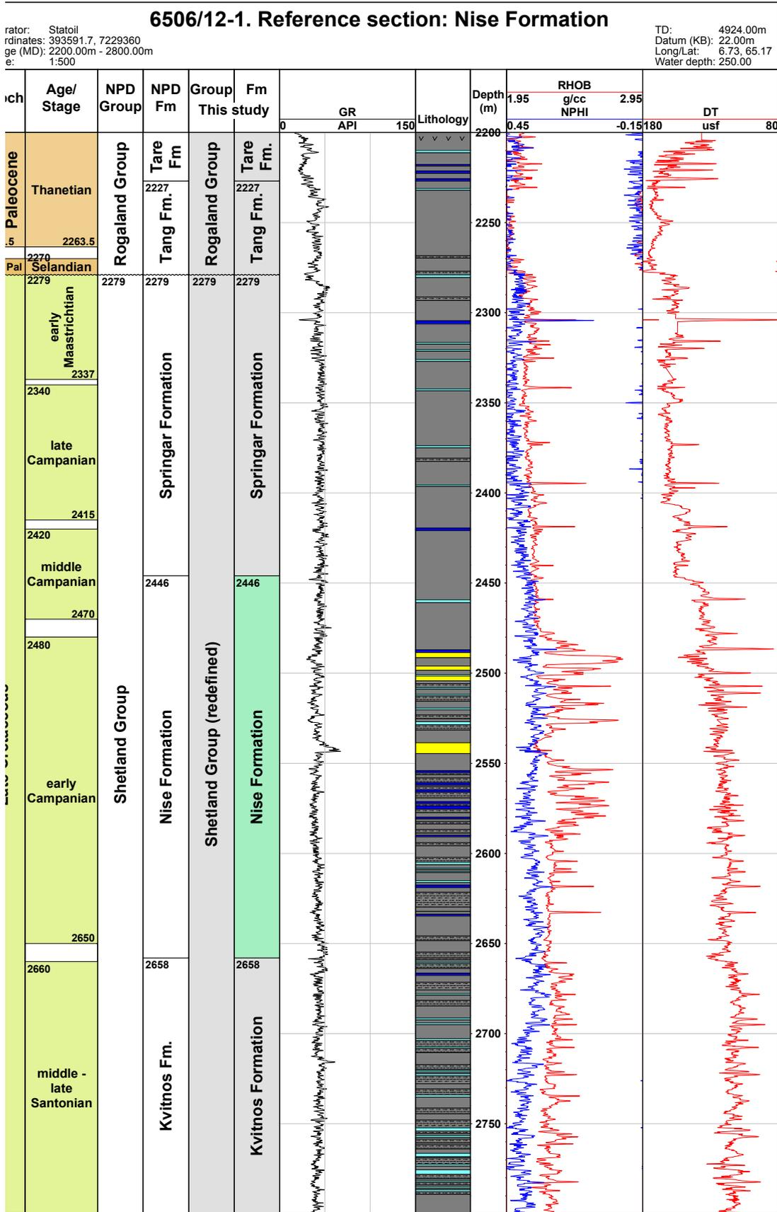
Figure 3.32. Well logs and lithology section for the Nise Formation in reference well 6506/12-1, Norwegian Sea.
