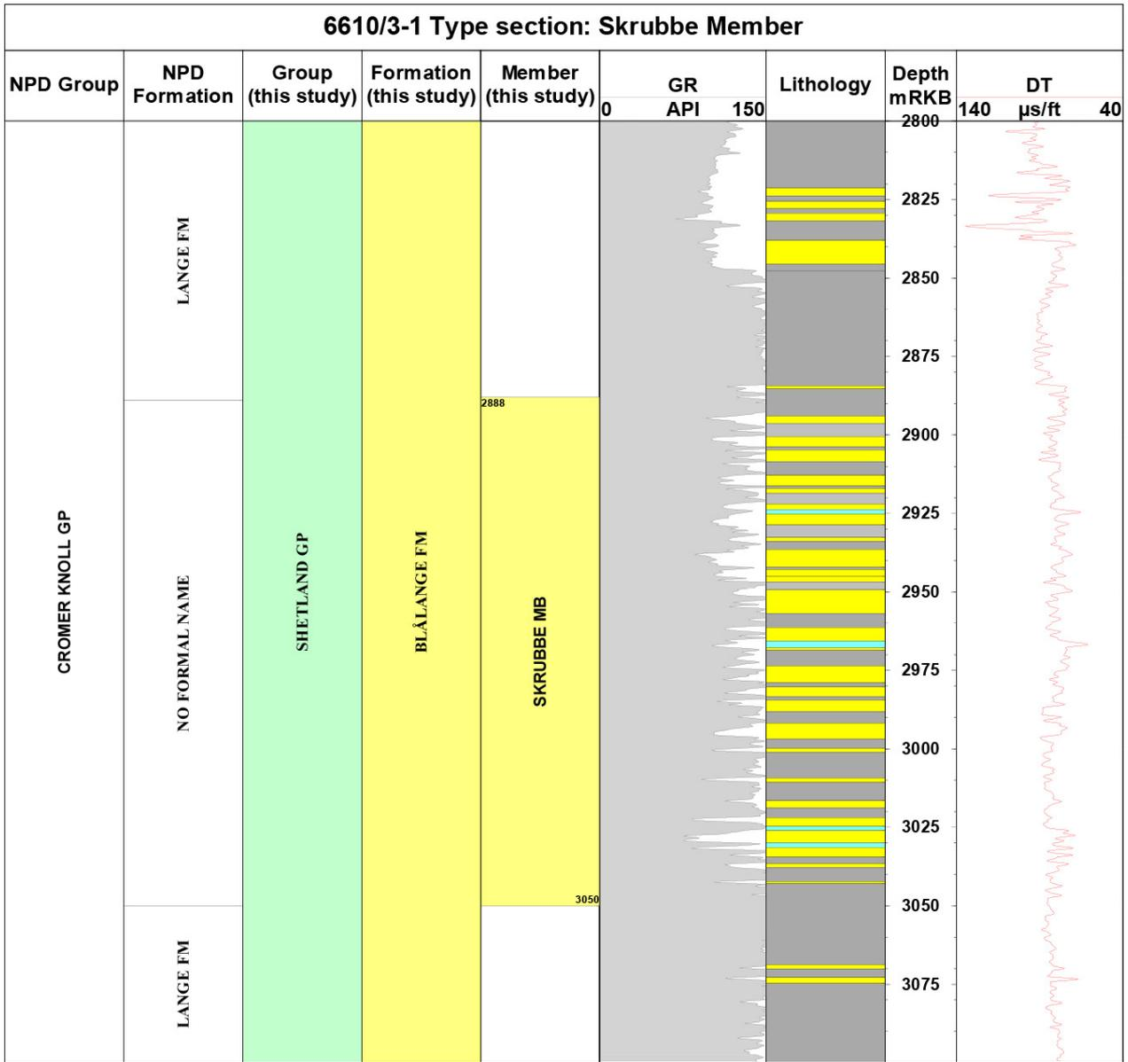
**Figure 3.19.** Well logs and lithology section for the Skrubbe Member of the Blålange Formation in type well 6610/3-1R, Norwegian Sea.
