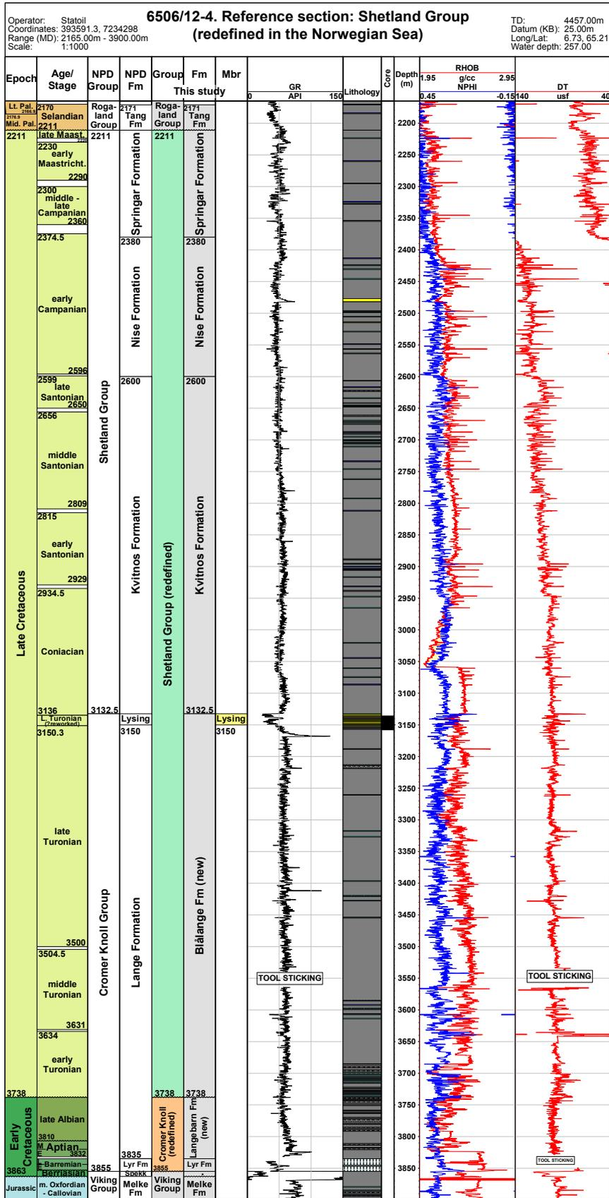
Figure 3.13. Well logs and lithology section for the Shetland Group in reference well 6506/12-4, Norwegian Sea.
