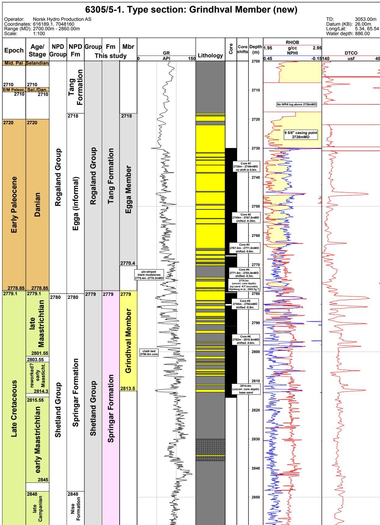
Figure 3.41. Well logs and lithology section for the Grindhval Member of the Springar Formation in type well 6305/5-1, Norwegian Sea.
