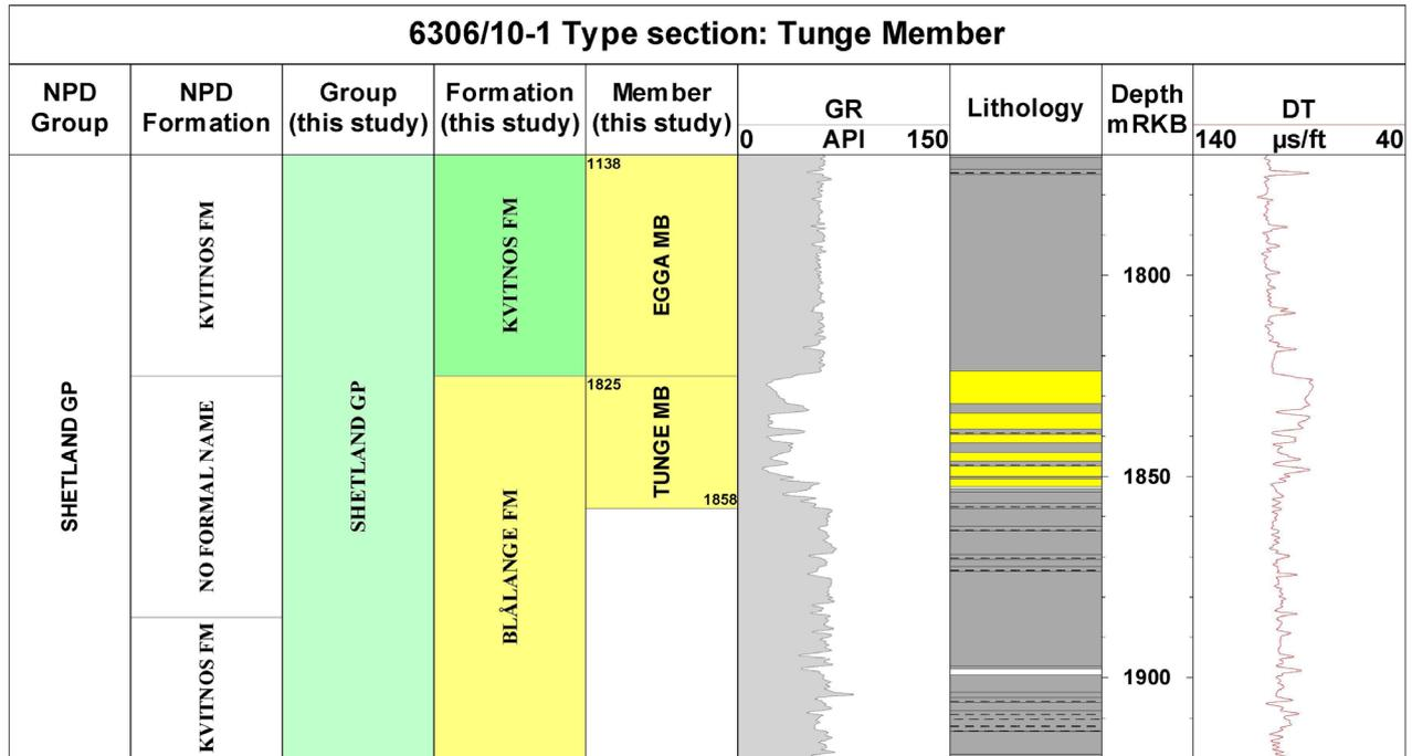
Figure 3.25. Well logs and lithology section for the Tunge Member of the Blålänge Formation in type well 6306/10-1, Norwegian Sea.
