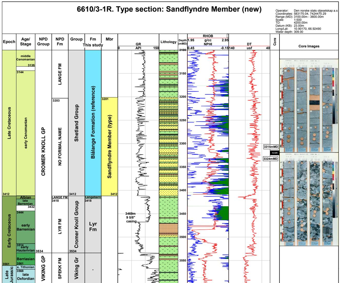
Figure 3.17. Well logs and lithology section for the Sandflyndre Member of the Blålange Formation in type well 6610/3-1R, Norwegian Sea.
