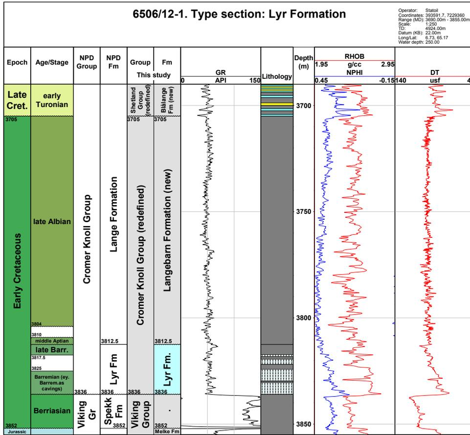
Figure 3.7. Well logs and lithology for the Lyr Formation in type well 6505/12-1, Norwegian Sea.
