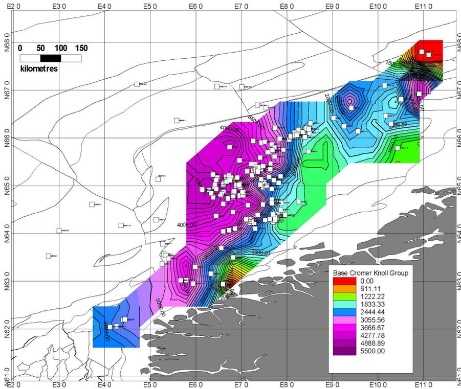
Figure 3.5. shows depth to the base of the Cromer Knoll Group (revised definition) in the Norwegian Sea based on released well data. The wells displayed are those that penetrated the base of the group.
