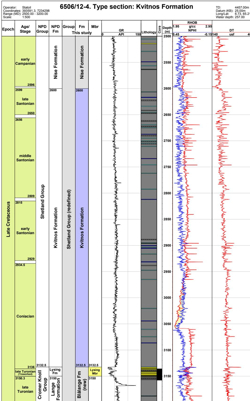
Figure 3.26. Well logs and lithology section for the Kvitnos Formation in type well 6506/12-4, Norwegian Sea.
