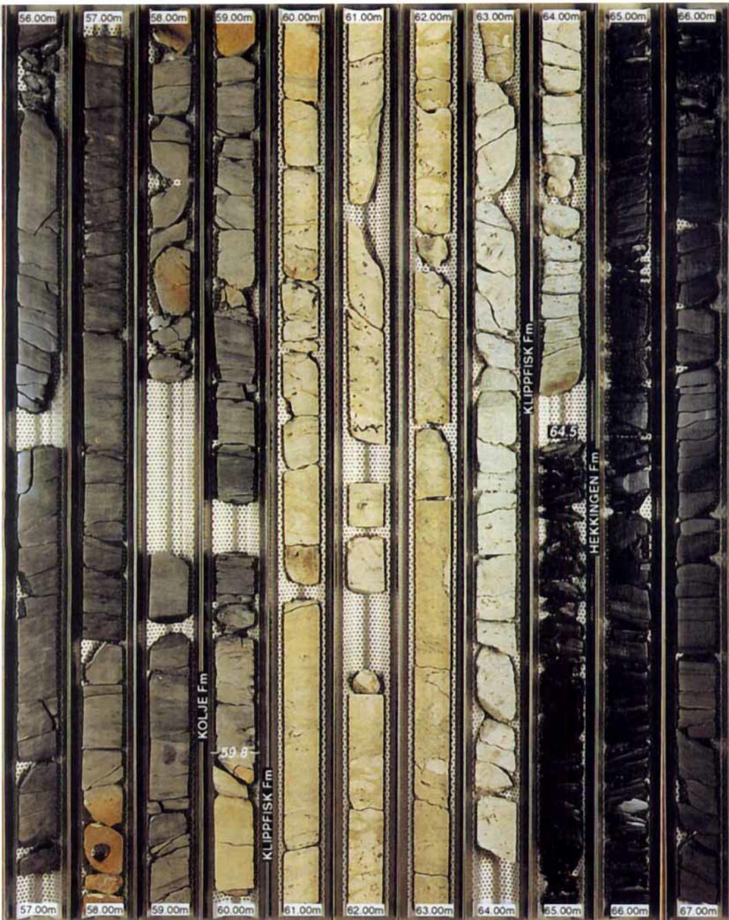
Fig. 4. Core photos from the Klippfisk Formation (Kutling Member) reference section in core 7231/01-U-01, Nordkapp Basin.
