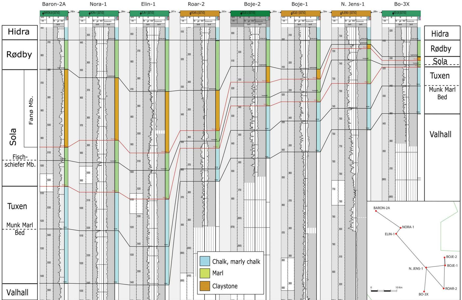
**Fig. A2.** Well-log correlation of the Lower Cretaceous displaying the lithostratigraphic units of the Cromer Knoll Group in the Danish Central Graben, including the new Fanø Member. Note the lateral variations in thickness of the Fanø Member, which is best developed in the centre of the basin. The red lines are sequence boundaries.
