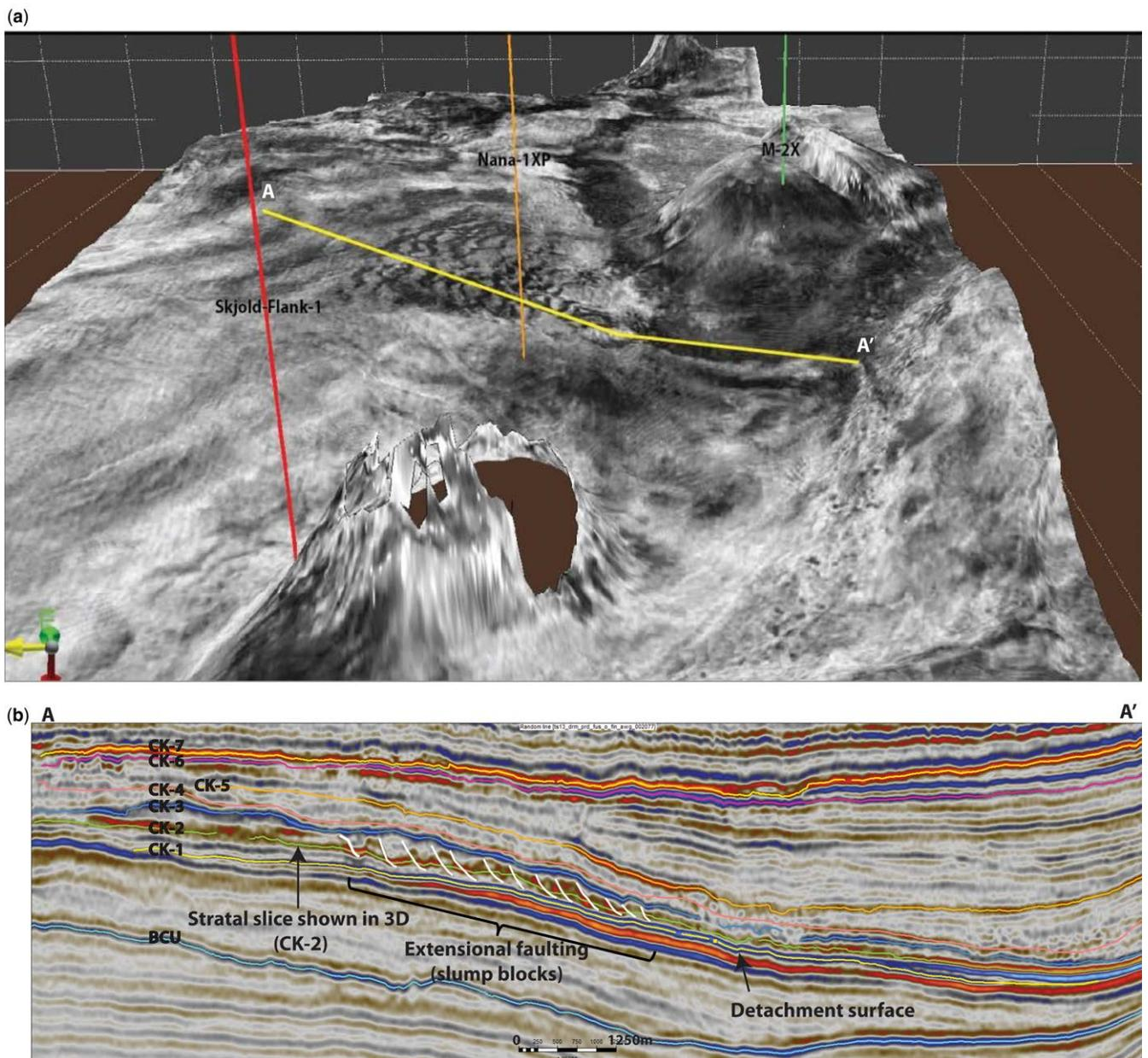
**Fig. 17.** Creep features in the Nana-1XP area. See Figure 16 for the location map: (a) 3D reconstructed geomodel horizon slice using a RMS amplitude, the position of the 2D line in (b) is indicated; and (b) 2D seismic line.
