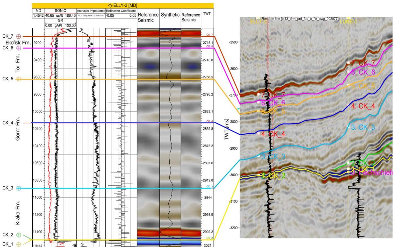
Fig. A5. Well log to seismic tie for the Elly-3 well. Note that the Hydra Formation and Roar Member are absent in this well. CK, seismic markers.
