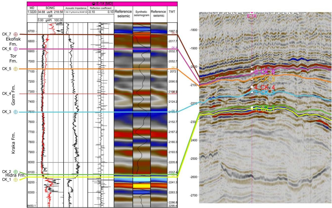
Fig. A4. Well log to seismic tie for the E-1 well. CK, seismic markers.
