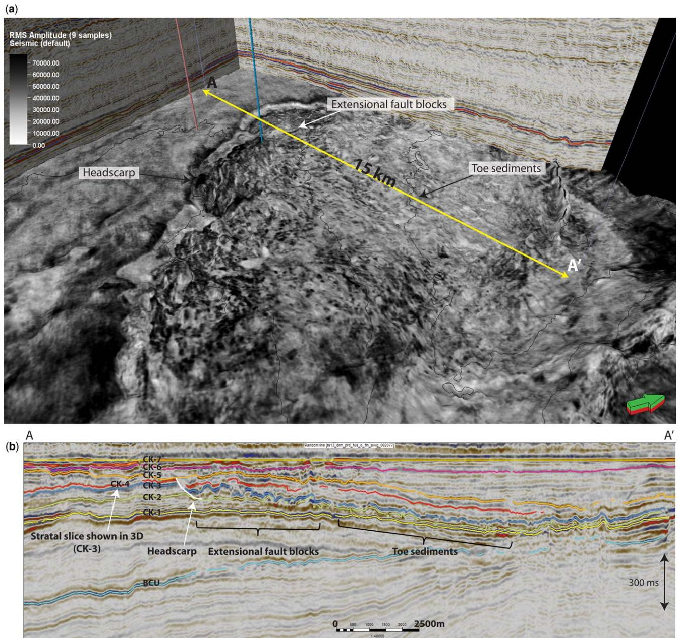
**Fig. 18.** Mass waste deposit in the Fasan-1 area. See Figure 16 for the location map: (a) 3D reconstructed horizon slice using RMS amplitude, the position of the 2D line used in (b) is indicated; and (b) 2D seismic line.
