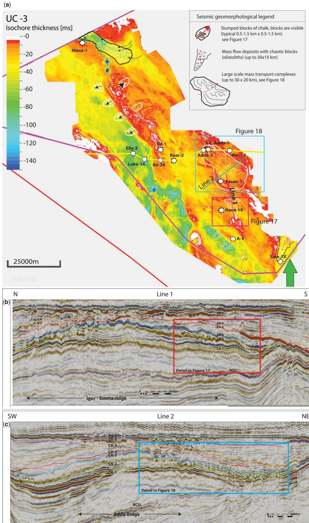
**Fig. 16.** Early-mid Campanian palaeotopography and gravity deposits: (a) Lower–middle Campanian isochore map, and distribution of slump, mass flows and mass-transport complexes; (b) seismic line 1, close to Nana-1X, showing slope destabilization in a southwards direction (see in detail in Fig. 17); and (c) seismic line 2, close to the Fasan-1 well, showing a large-scale mass-transport complex along the eastern margin of the inverted high (see in detail in Fig. 18).
