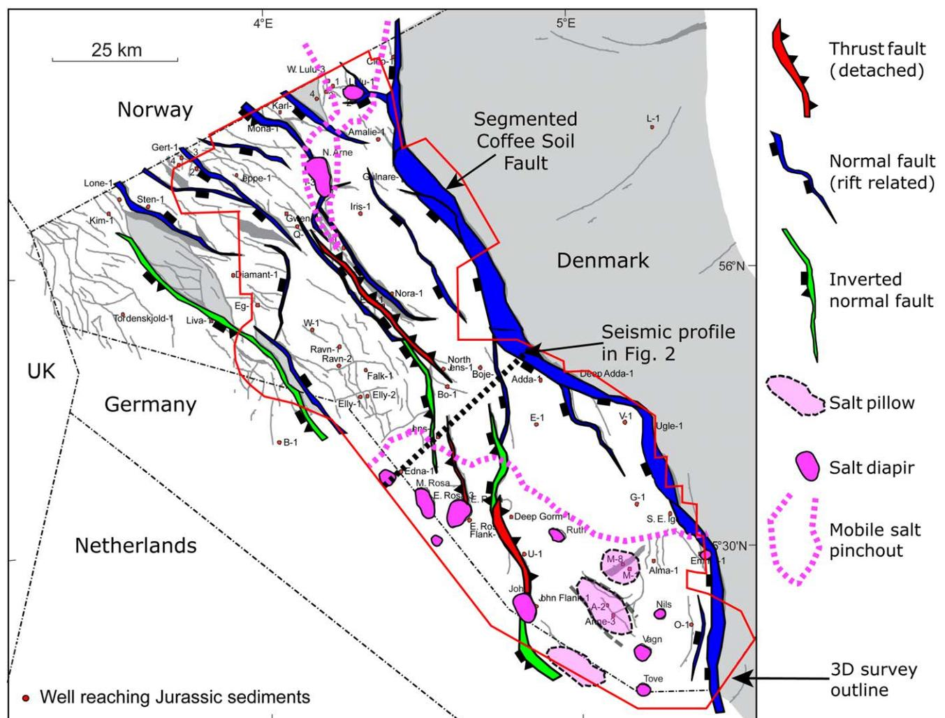
Fig. 1. Structural elements map of the Danish Central Graben (modified after Japsen *et al.* 2003). The aerial extent of the seismic survey used is indicated.
