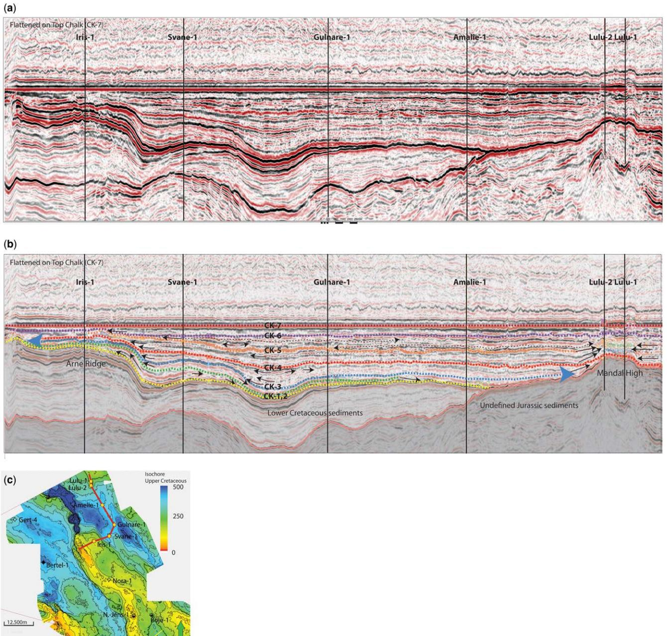
**Fig. 6.** Seismic cross-section in the northern part of the Danish Central Graben flattened on the top of the Chalk Group. (a) Seismic line. (b) Interpreted seismic line. Note the onlap of the Campanian and Maastrichtian deposits (between seismic markers CK-3 and CK-6) against the Arne Ridge. (c) Position of the seismic transect shown on the Upper Cretaceous isochore map.
