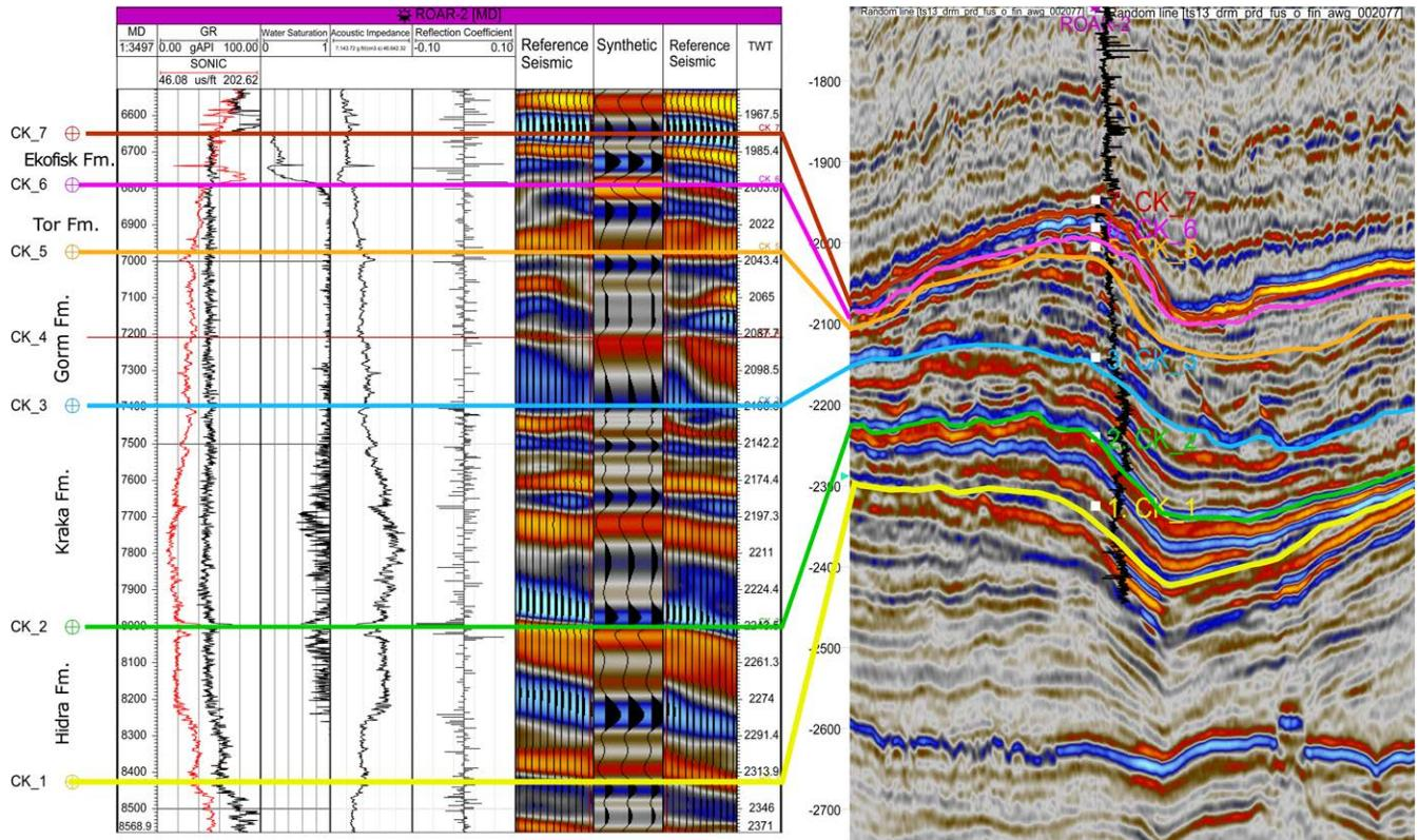
**Fig. A6.** Well log to seismic tie for the Roar-2 well. CK, seismic markers.
