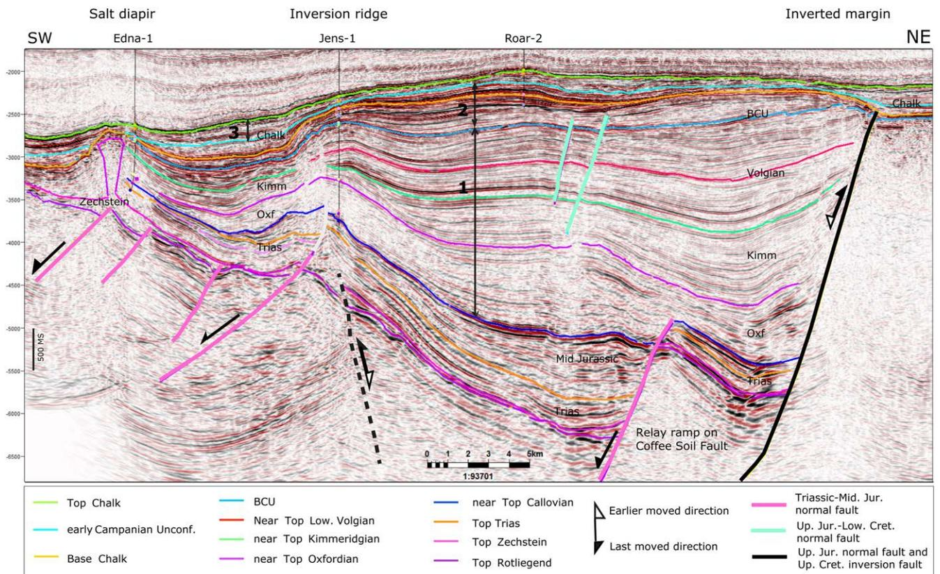
**Fig. 2.** East-west structural cross-section of the Danish Central Graben illustrating the Late Jurassic rift phase (1), the Cretaceous–Cenozoic thermal subsidence post-rift phase (2) and the Late Cretaceous basin inversion event (3). See Figure 1 for the location map. In this 2D transect, reactivation of a deep-seated normal fault is proposed to explain the inversion-related anticlinal structure in the Jens-1 location.
