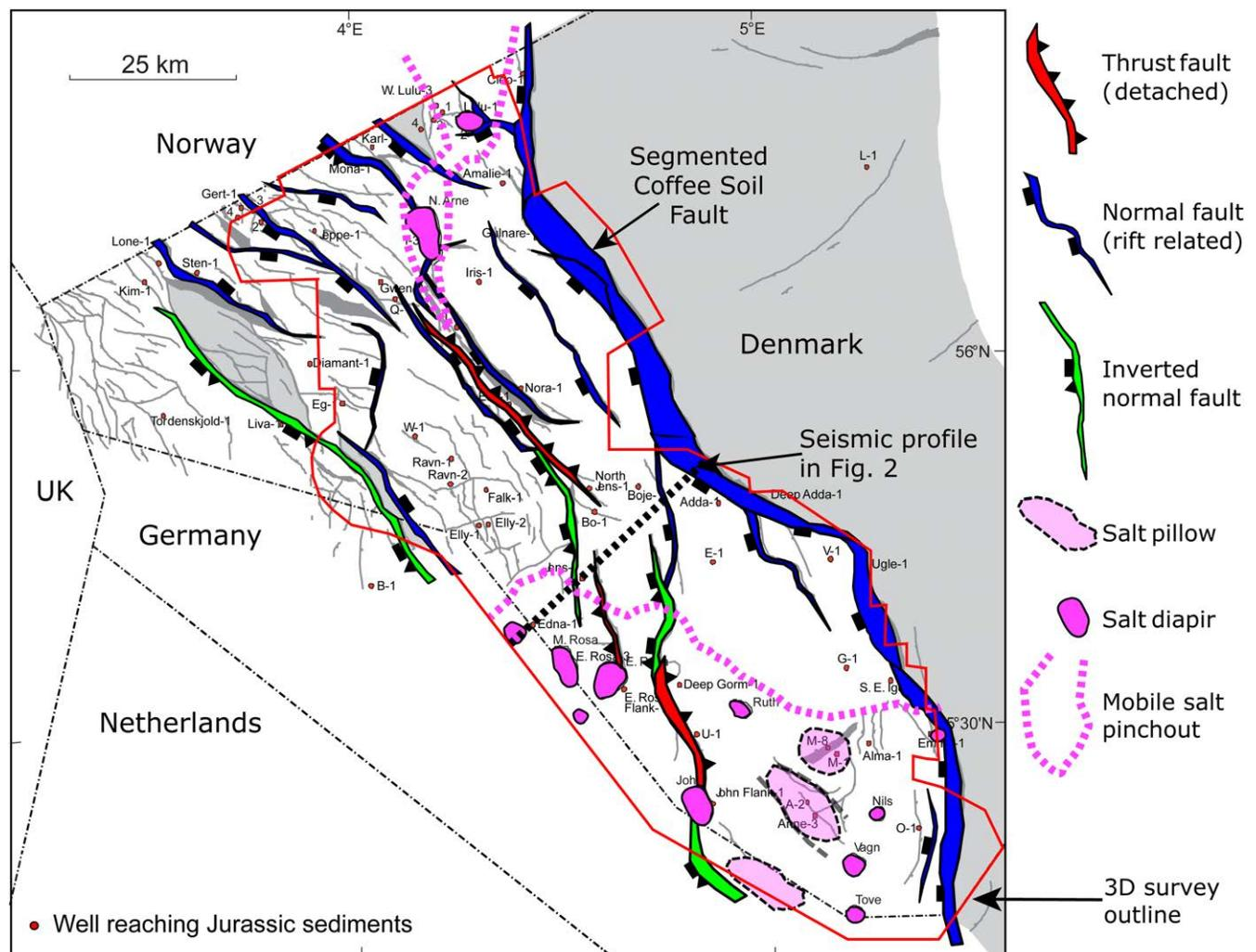
**Fig. 1.** Structural elements map of the Danish Central Graben (modified after Japsen *et al.* 2003). The aerial extent of the seismic survey used is indicated.
