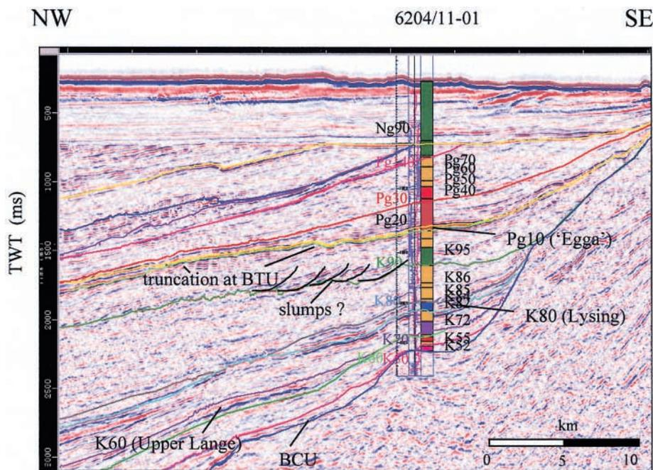
**Fig. 3.** Example of seismic line with well, Møre Basin, showing the Cretaceous–Tertiary succession. Note the higher frequency of sequences in the well compared to the seismic events, and high seismic amplitudes in sandstone-bearing sequences Pg10–20, K80, K60. Seismic data courtesy of TGS-NOPEC Geophysical Company. See Figure 1 for location.
