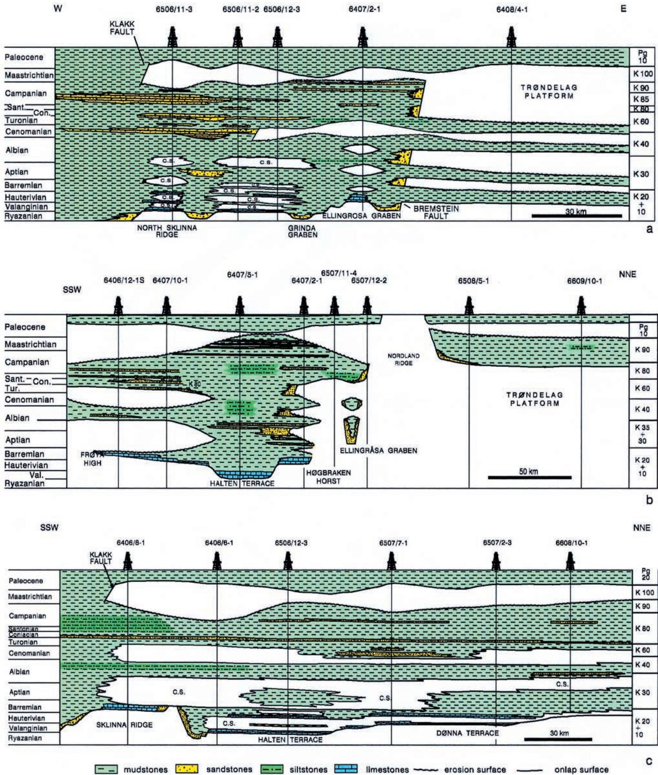
Fig. 5. Chronostratigraphic well correlations: (a) across the Halten Terrace; (b) along the Halten Terrace and Trøndelag Platform; and (c) along the Halten and Donna terraces. For location of wells see Figure 1. Time-scale in Figure 4.
