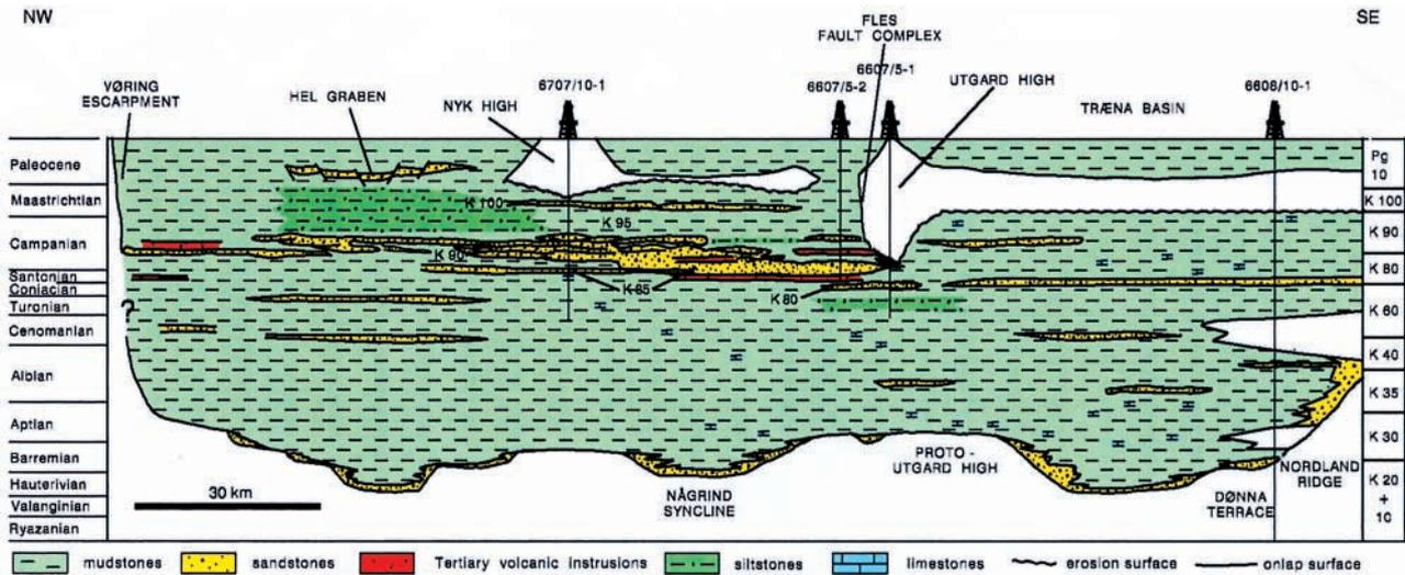
Fig. 6. Chronostratigraphic well correlation, Vøring Basin. For location of wells see Figure 1. Time-scale in Figure 4.
