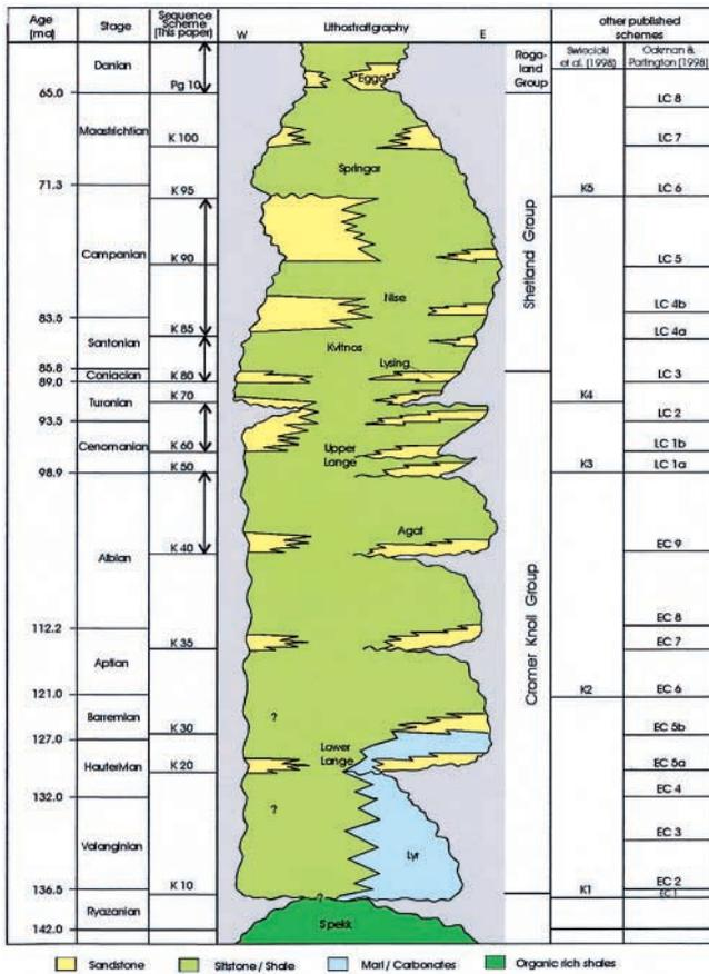
Fig. 4. Stratigraphic summary of Cretaceous sequences and formations with equivalencies to other schemes. Time-scale after Gradstein & Ogg (1996); stratigraphy of east portion based mostly on Dalland *et al.* (1988) and of west portion on data from Brekke *et al.* (1999), except position of the Nise equivalent sandstones, which is based on our own results from the Nyk High well.
